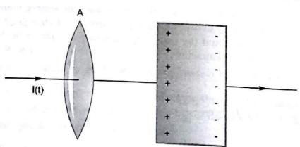
During charging C capacitor, a time varying current I(t) flows through the conducting wire, so on applying Ampere's circuital law (for loop A)  $\oint \overrightarrow{B} \cdot \overrightarrow{dl} = \mu_o I(t)$
